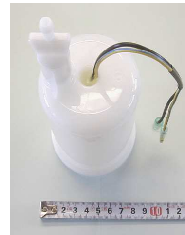
Sensor Ass'y ( Fuel filter )
